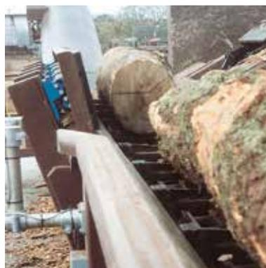
Dampening of an **impact bed** for logs
