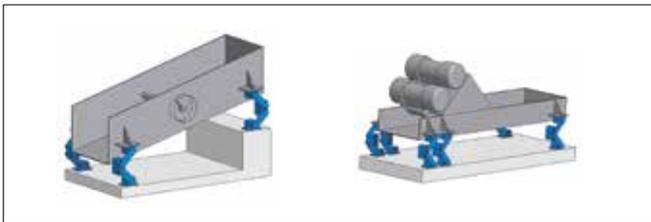
Plants with eccentric drives are ideal for mining, quarries and much more. Thanks to ROSTA, the high forces generated at the start-up and especially when shutting down, are quickly and effectively absorbed.
