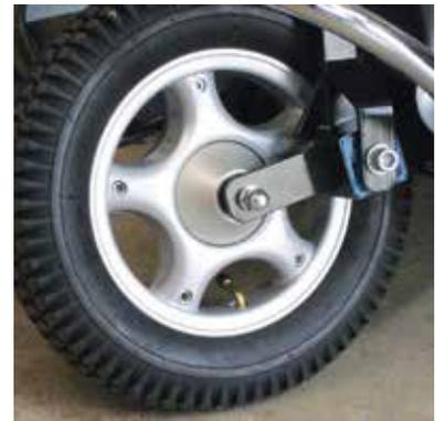
Rubber suspension for the **wheel suspension**
