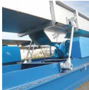
Conveying and screening trough for **wood splinters**
