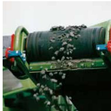
Suspension for **belt scrapers** on conveyor belts
