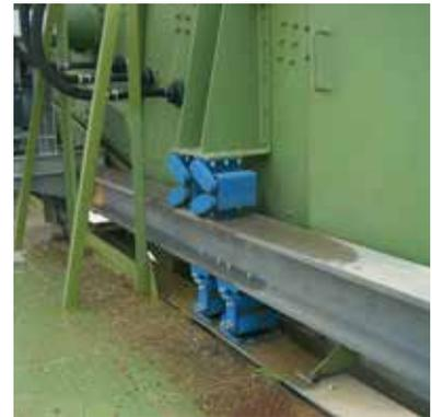
**Counter-oscillating frame mounting** for a vibrating screen
