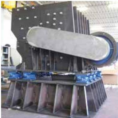
Vibration damper for **recycling crushers**
