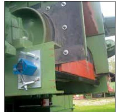
Rubber suspension element for **conveyor belt scrapers**
