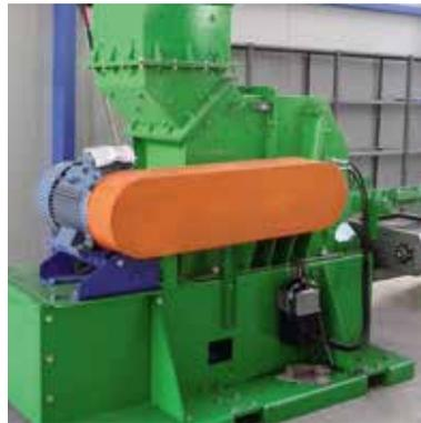
Motor base in a chipper for the recycling industry
