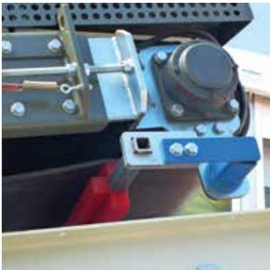
Tensioner device for **conveyor belt scrapers**
