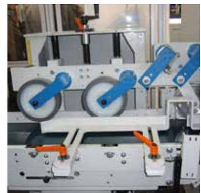
Tensioner devices with **hold-down rollers**
