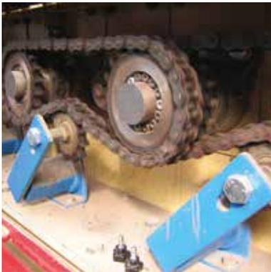
Tensioner devices for chain drives on loading stations
